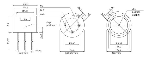
GaP blue light detector with integrated amplifier
